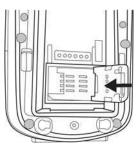
5. Close the cover over the slot, and then slide the cover to the left to lock the SIM card.
