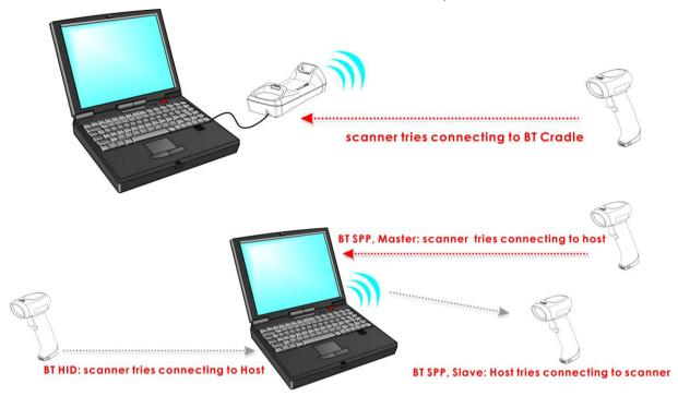
Note: If RS-232, USB Virtual COM or BT SPP is selected for output interface, the host can directly send serial commands to configure the scanner. For example, run HyperTerminal.exe and type the 6-digit command located under each setup barcode. Refer to <a href="#">Appendix II Host Serial Commands</a>.
